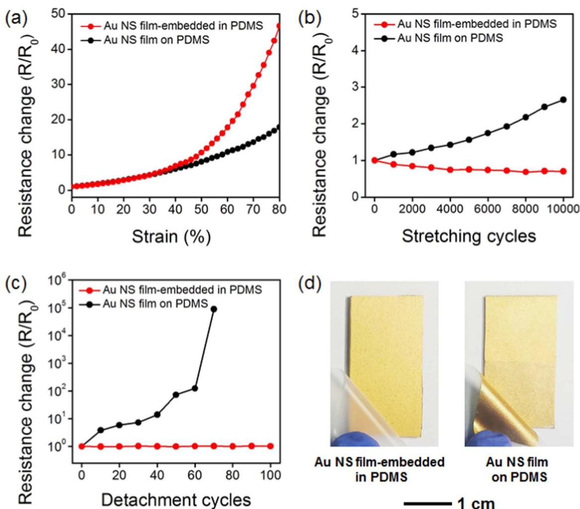
Fig. 2. (a) Change in resistance ( $R/R_0$ ) for Au NS electrodes in response to tensile strain. (b) Variations of  $R/R_0$  for Au NS electrodes during 10,000 cycles of stretching at a 30% strain. During the cycles, the resistance was measured after the releasing of the strain. (c) Variations of  $R/R_0$  for Au NS electrodes during 100 cycles of the Scotch-tape detachment test. (f) Photographs showing the tape-contact regions of Au NS electrodes after the detachment test.
