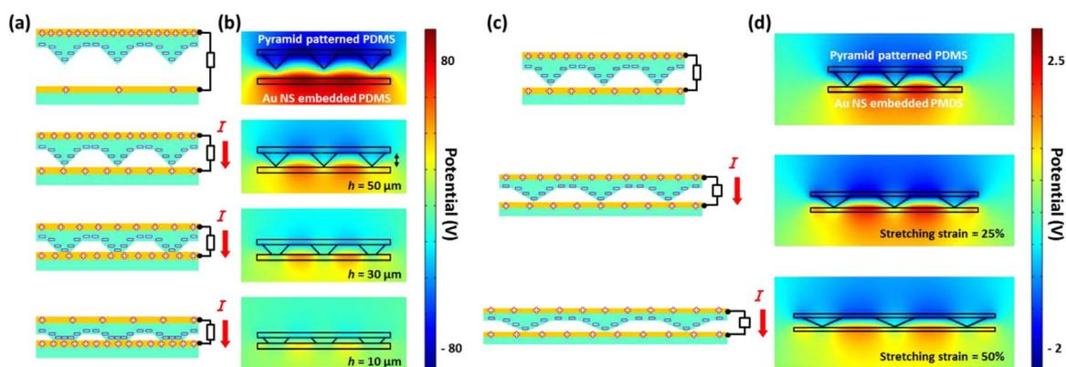
Fig. 3. Schematic illustration of the working mechanism and finite-element simulation of the generated voltage difference of the Au NS-TENG in the (a–b) vertical and (c–d) horizontal motions.
