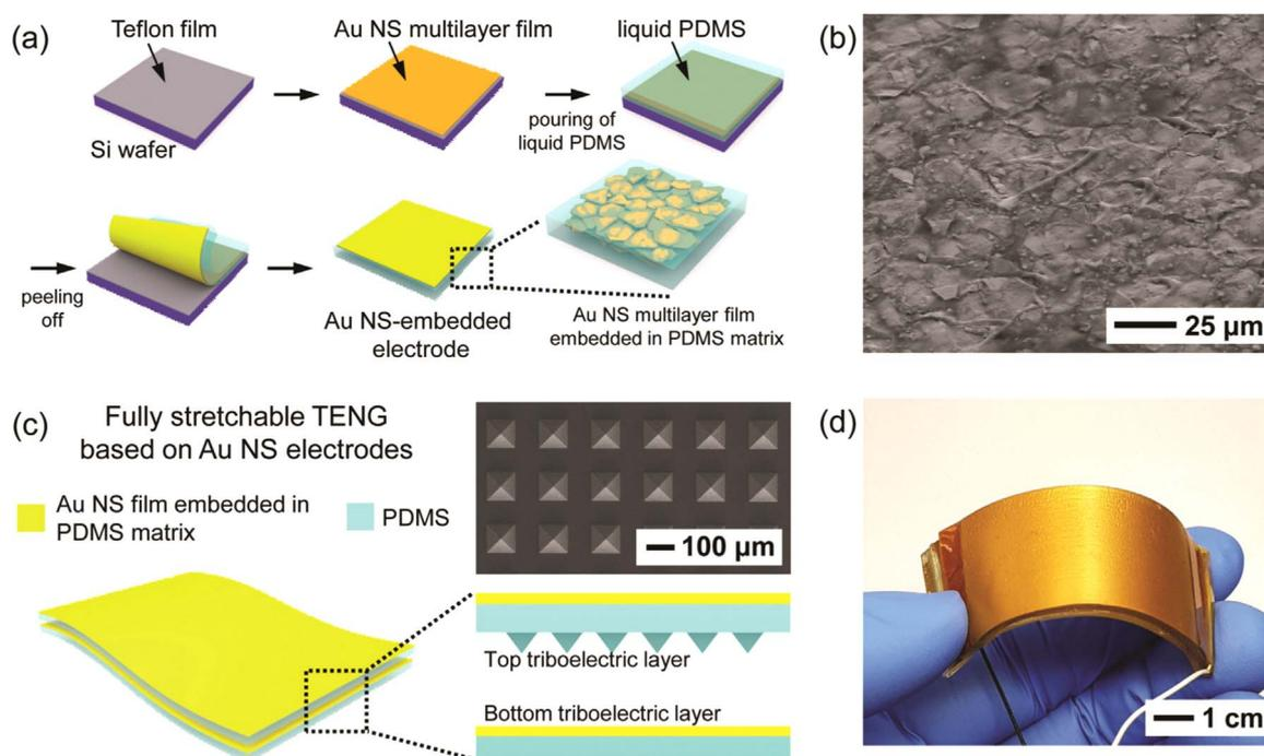
**Fig. 1.** (a) Schematic illustration of the fabrication process of the Au NS-embedded electrode. (b) Top-view FE-SEM image of the Au NS-embedded electrode. (c) Schematic illustration of the structure of the fully stretchable TENG based on the Au NS-embedded electrodes. The FE-SEM image shows the micropyramid-patterned PDMS (10  $\mu\text{m}$  width) of the top triboelectric layer of the TENG. (d) Photograph of the Au NS-TENG.
