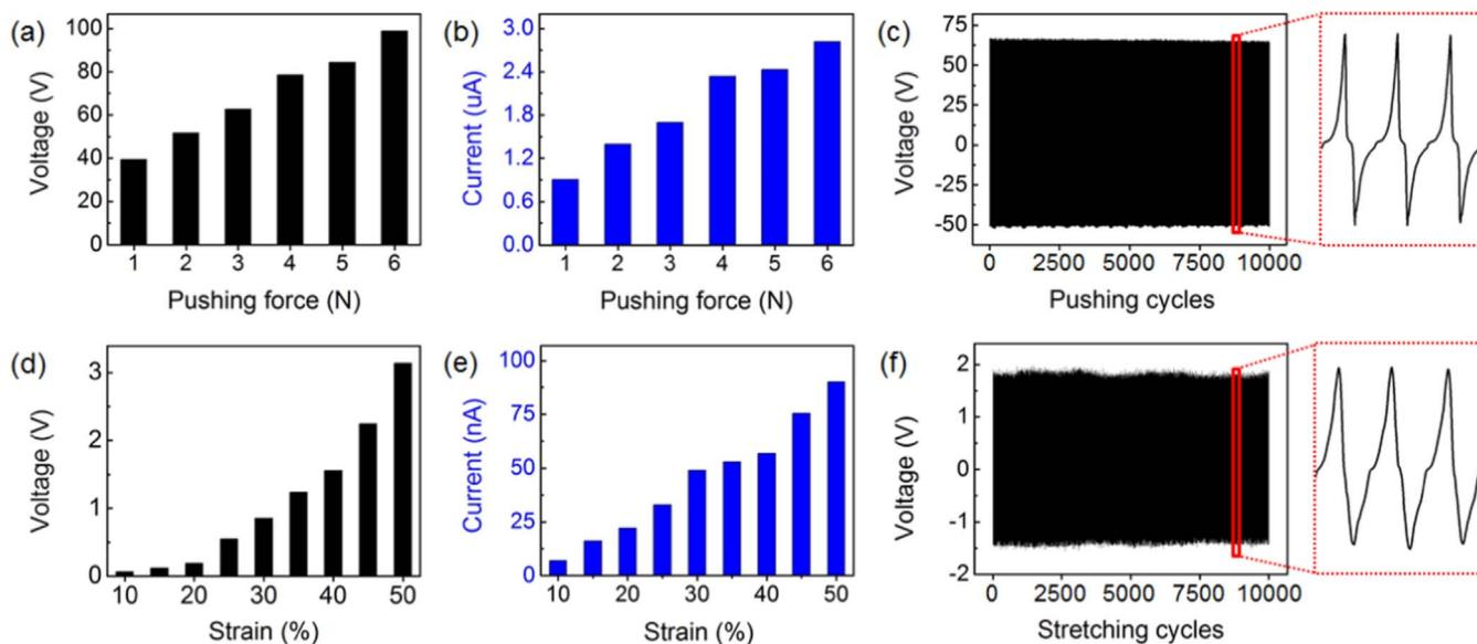
Fig. 4. Output performance of the Au NS-TENG. Voltage output, current output, and durability tests during the 10,000 cycles in the (a–c) pushing mode of the vertical direction and the (d–f) stretching mode of the horizontal direction.
