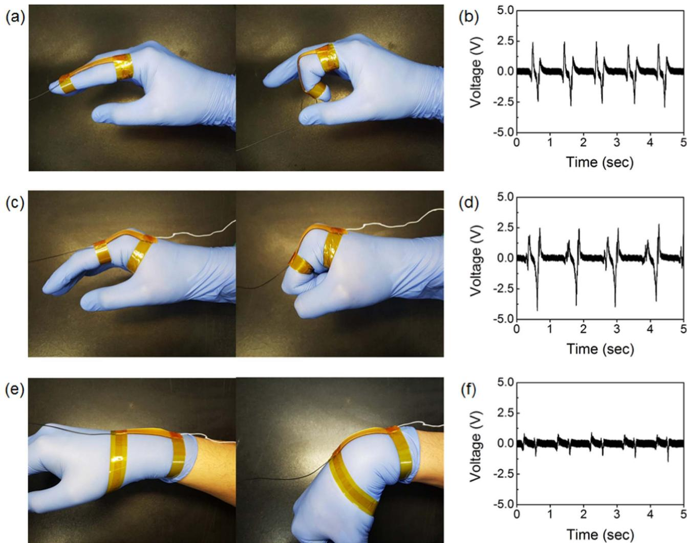
Fig. 5. Photographs and output-voltage responses to the repeated bending/relaxation of the Au NS-TENG that was mounted on the (a, b) index finger, (c, d) knuckle, and (e, f) wrist, respectively.
