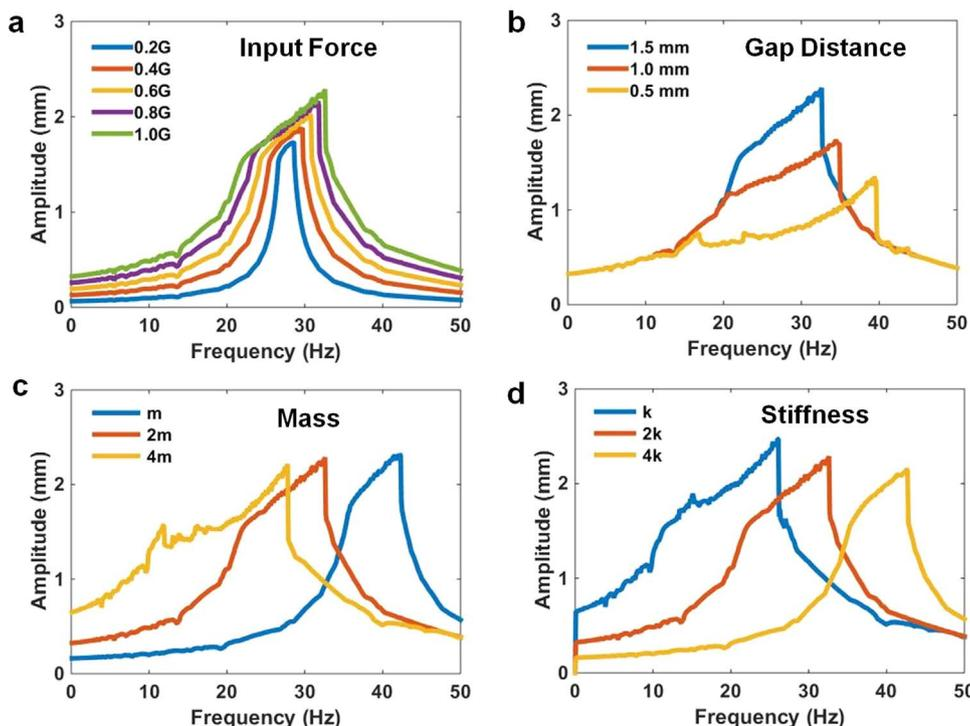
Fig. 2. Understanding of coupling effect for control parameters of VTENG via simulation. Amplitude response of VTENG when changing (a) input acceleration, (b) separation gap distance between the tribo-active materials, (c) moving mass, and (d) spring stiffness.
