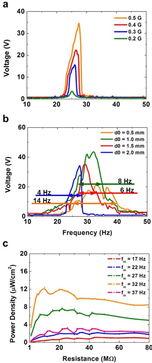
**Fig. 3.** Experimental investigations for critical control parameters of VTENG. Peak voltage response of VTENG when changing the (a) input acceleration and (b) separation gap distance ( $d_0$ ) between the tribo-active materials. (c) Output power density curves at different input frequencies according to the load resistance, for  $d_0 = 1$  mm.
