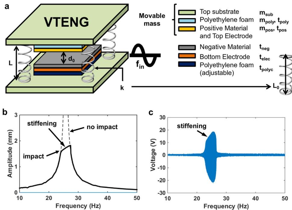
Fig. 1. Control parameters and resonant output behavior for VTENG. (a) Schematic of VTENG showing important design parameters. (b) Amplitude response simulation stiffening characteristic under impact condition. (c) Resonant output voltage response of VTENG with stiffening.
