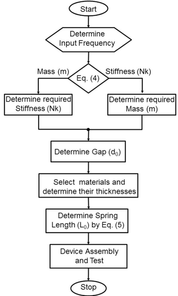
**Fig. 4.** Resonant design protocol for optimization of an individual VTENG. The design protocol is based on a modified vibration theory for maximizing the power output of the VTENG.
