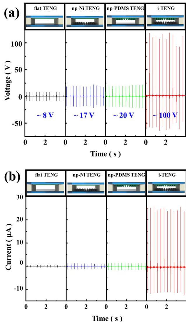
Fig. 4. Output (a) voltages and (b) currents for four different types of TENG devices.
