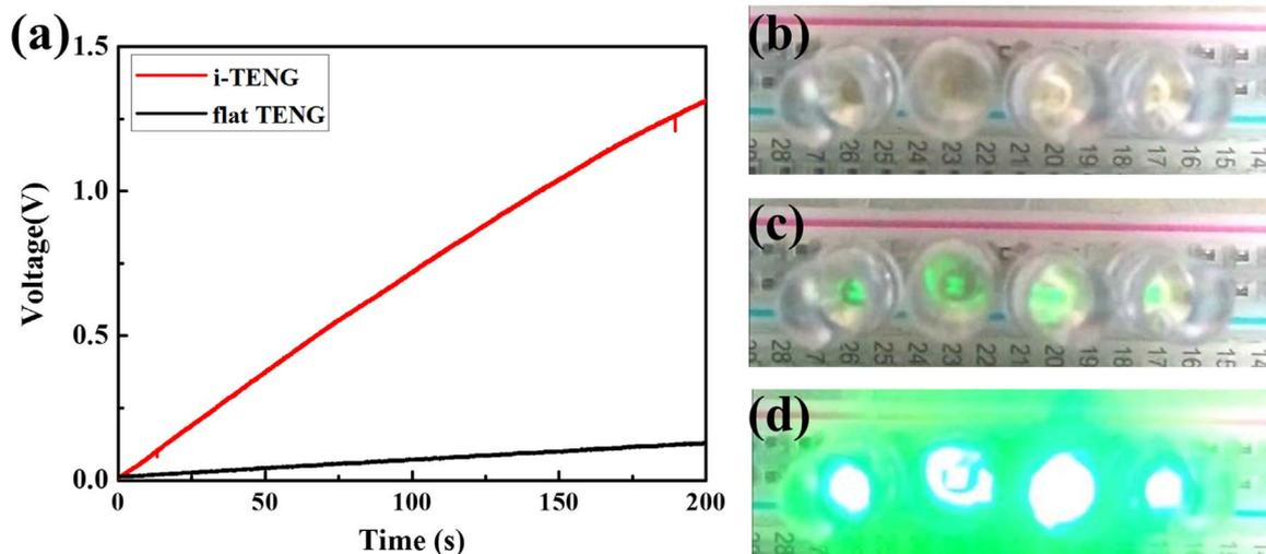
**Fig. 6.** (a) Charging characteristics of commercial capacitor based on output electricity generated by flat TENG and i-TENG with vibration of 10 Hz. Charging characteristics of commercial capacitor based on output electricity generated by flat TENG and i-TENG with vibration of 10 Hz. Discharging process for charged capacitor used for LED lighting: (b) setup state, operating state; (c) capacitor charged by flat TENG; and (d) i-TENG.
