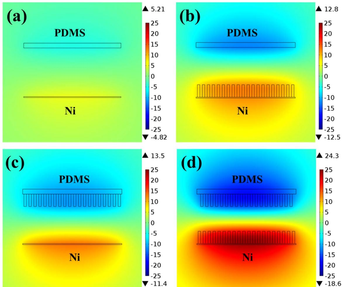
Fig. 2. Finite element simulation of vertical contact-separation modes for four different kinds of TENGs using COMSOL Multiphysics software: (a) flat TENG, (b) np-Ni TENG, (c) np-PDMS TENG, and (d) i-TENG.
