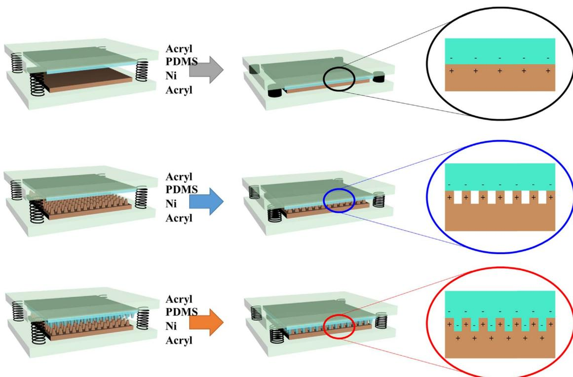
Fig. 3. Working principles for (a) flat TENG, (b) np-Ni or np-PDMS TENG, and (c) i-TENG.
