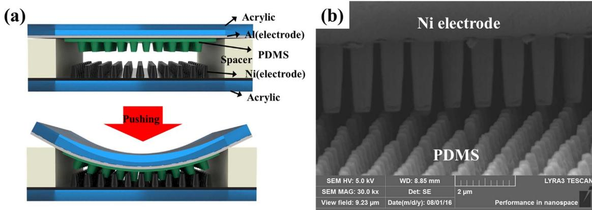
Fig. 1. (a) Schematic illustration and (b) SEM micrograph of i-TENG.
