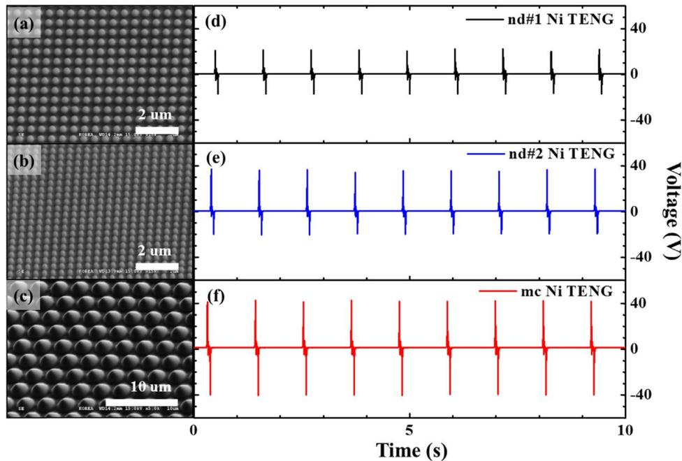
**Fig. 5.** SEM micrographs of (a) nano-dot#1 Ni, (b) nano-dot#2 Ni, and (c) micro-cone Ni electrodes and output voltages of (d) nd#1 Ni TENG, (e) nd#2 Ni TENG, and (c) mc Ni TENG.
