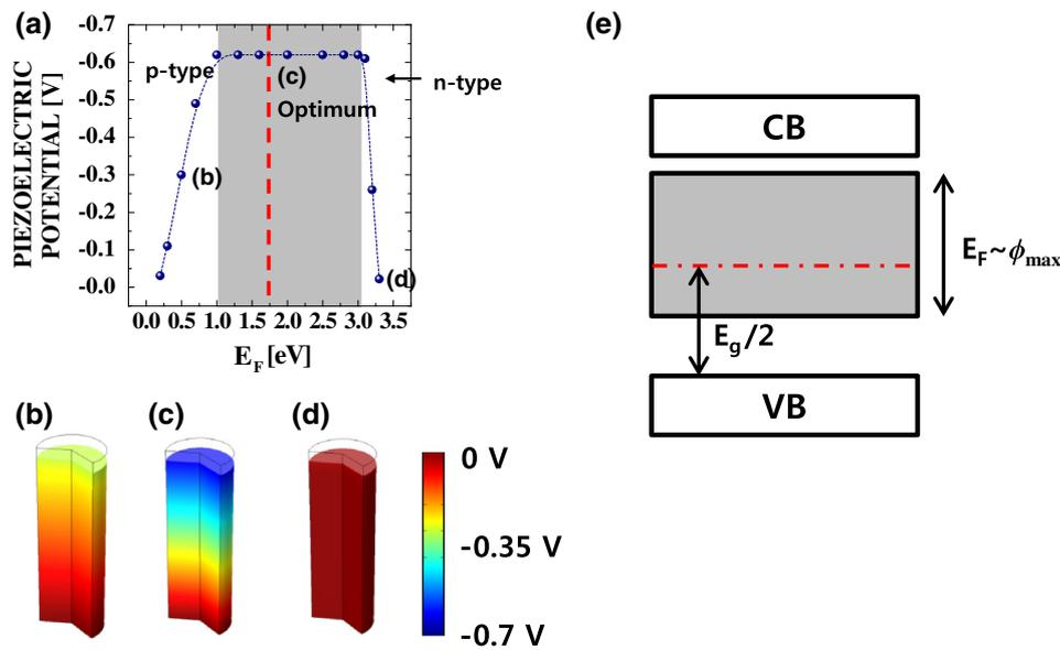
**Fig. 2 a** Piezoelectric potential calculated at the top surface of the ZnO NWs under uniaxial compression as a function of the equilibrium Fermi level ( $E_F$ ). At each side of region, it can be seen that the piezoelectric potential is significantly reduced due to the free-carrier screening effects. **b–d** Piezoelectric potential distribution along the  $z$ -axis corresponding to each point of the main plot. The
