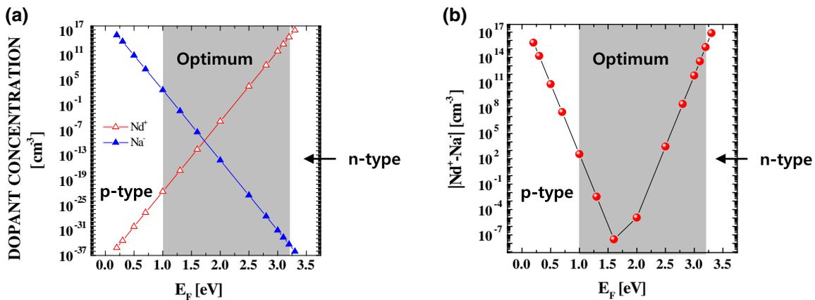
**Fig. 4** **a** Calculated ionized donor ( $N_d^+$ ) and ionized acceptor ( $N_a^-$ ) concentrations as a function of  $E_F$  with a neutrality condition of  $-n + p = N_a^- - N_d^+$ . Note that the shaded area indicates the optimum region where the maximum piezoelectric potential is maintained as seen in Fig. 2a. **b** Calculated dopant difference between  $N_d^+$  and  $N_a^-$ , which approaches zero near the mid-gap within the optimum range
