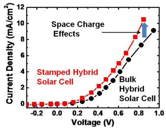
**Figure 4.** Dark current–voltage characteristics for both the stamped and bulk hybrid cells. It can clearly be observed that the bulk hybrid cell follows the space–charge–limited current at higher forward biasing.
