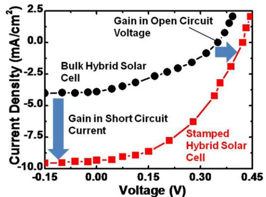
**Figure 5.** Illuminated current–voltage characteristics for both cells under AM1.5G illumination for photovoltaic measurement, where the stamped hybrid solar cell shows significant improvement in short-circuit current and open-circuit voltage.
