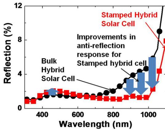
**Figure 3.** Optical reflectance spectra for the stamped and bulk hybrid solar cell. The bulk hybrid cell shows slightly enhanced anti-reflection for the wavelength range of 300–700 nm, but the anti-reflection above 700 nm is very significantly enhanced for the stamped hybrid solar cell compared with the bulk hybrid cell.
